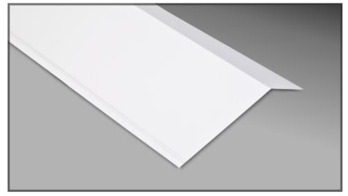
Manufactured of.019" aluminum and painted on Englert's state of the art coil coating line. Englert Drip Edge is available in 6" and 4" sizes and comes in 10' lengths. Available in white and brown. Packaged 30 per box.
