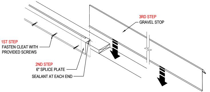
STEP 1, INSTALL 22 GA. GRAVEL STOP CLEAT WITH PROVIDED SCREWS FROM MANUFACTURER. INSTALLED 12" O.C. AND MAKE SURE TO ADD SEALANT AT SEAMS.
